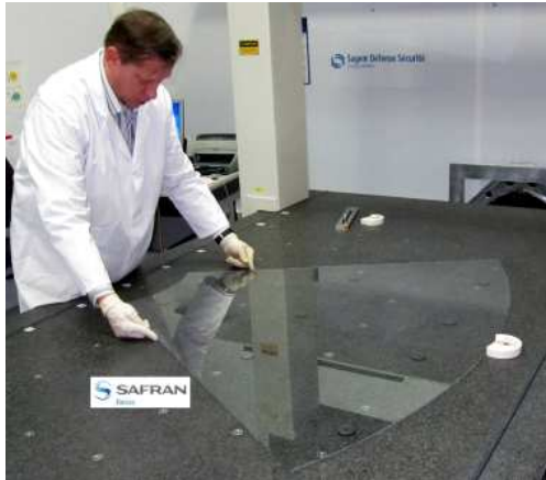
Fig. 5. Prototype of one of the 6 glass ceramic thin-shell petals to constitute the future M4 adaptive optics deformable mirror (2.4-m diameter and 1.95-mm thick).
